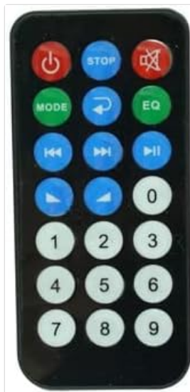
Figure 1: Front view of the remote control. This image displays the layout of all functional buttons, including power, mode selection, playback controls (play/pause, skip), volume adjustments, equalizer (EQ), mute, and a numeric keypad.
