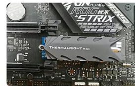
M.2 2280 PRO after installation
