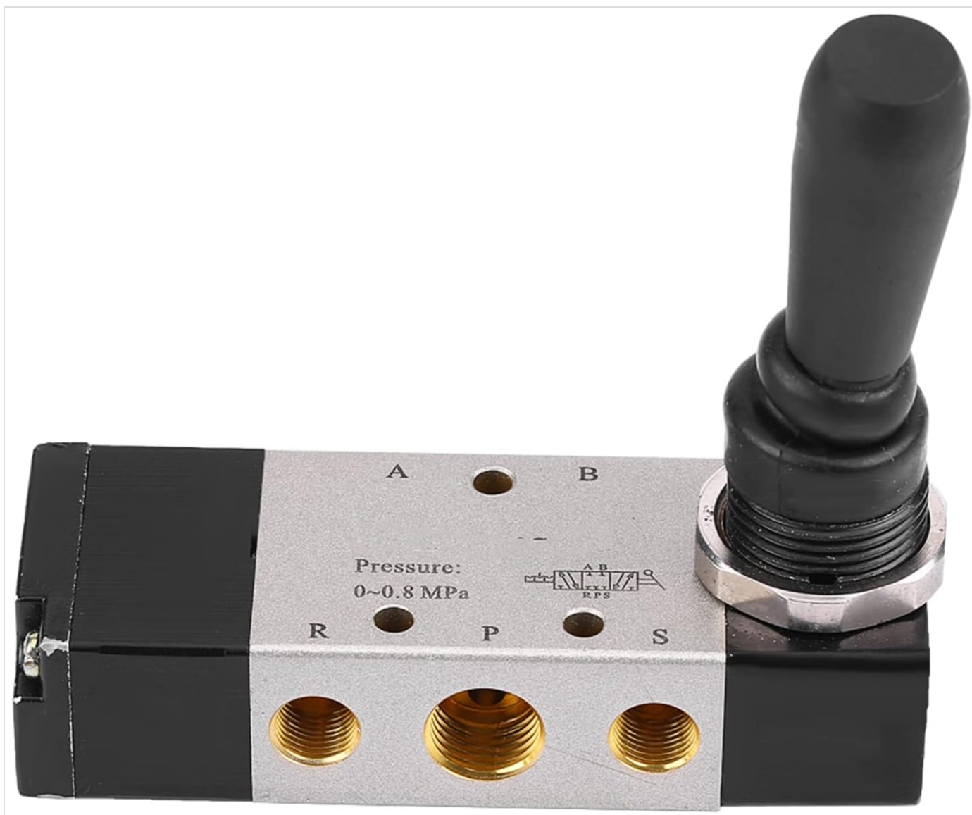
Figure 2.2: Top view of the valve, highlighting the air connection ports (P, A, B, R, S). The 'P' port is for pressure input, 'A' and 'B' are working ports, and 'R' and 'S' are exhaust ports, typically connected to mufflers. This view clearly shows the labeling for each port.
