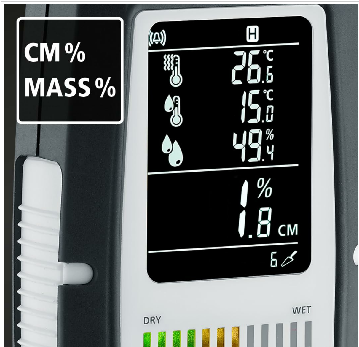
Figure 4: The device's display showing readings in "CM%" or "MASS%" mode. This view provides specific moisture content percentages, alongside the ambient condition readings.
