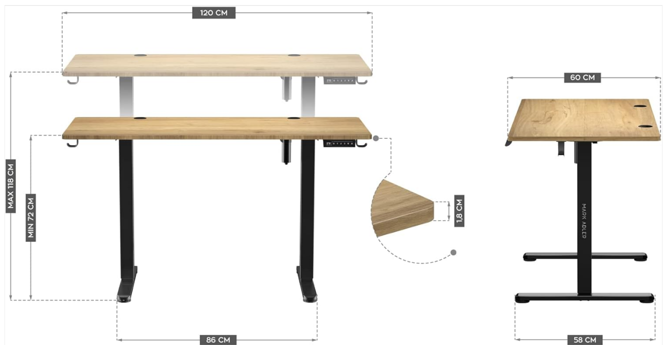
Figure 1: Desk Dimensions and Height Range
