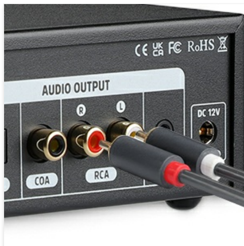
Figure 5: Connecting RCA audio cables to the DP01.
