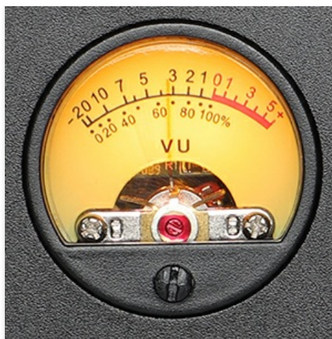
Figure 10: The dynamic VU level meter provides a visual representation of audio levels.
