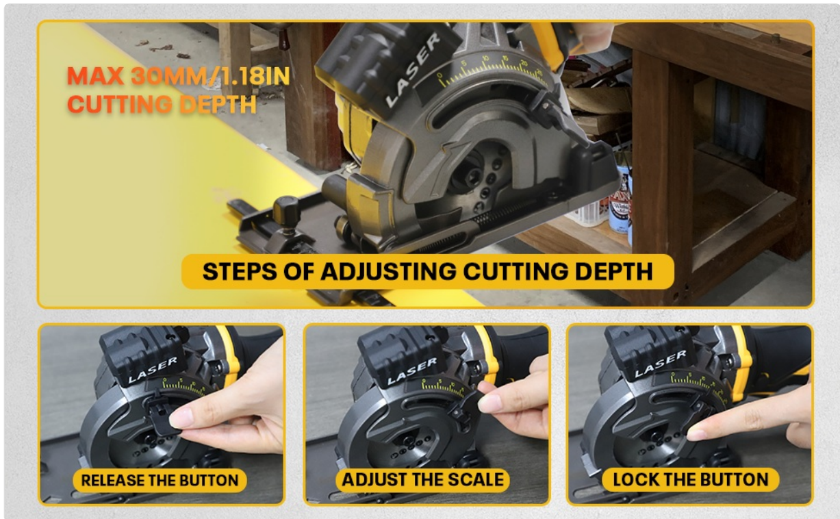
Figure 3.3: Follow these steps to adjust the cutting depth accurately.
