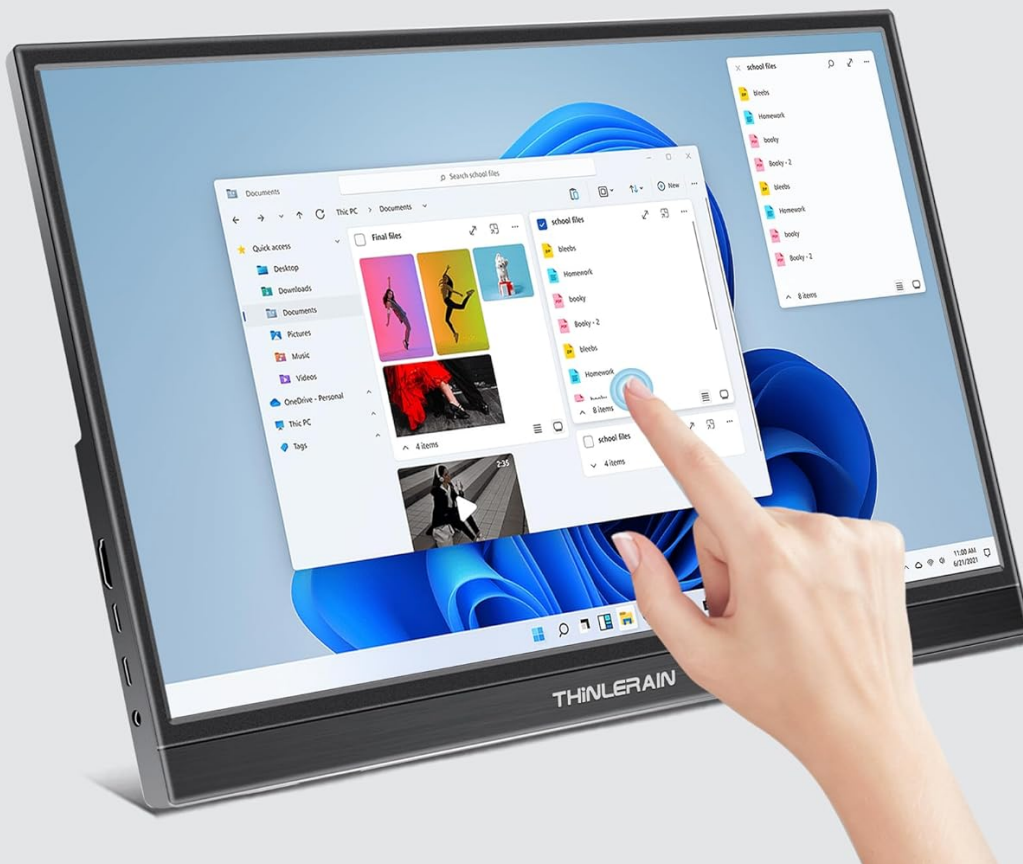
Image 4.2: Ten Point Touch Screen. This image illustrates the monitor's ten-point touch capabilities, showing various gestures like touch, enlarge, zoom out, drag, whirligig, and two-finger touch, with a hand interacting with a Windows desktop environment.
