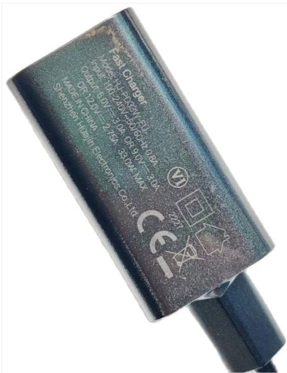
Image 3: A close-up view of the GEPA33W Fast Charger, displaying its technical specifications and certifications on the casing.
