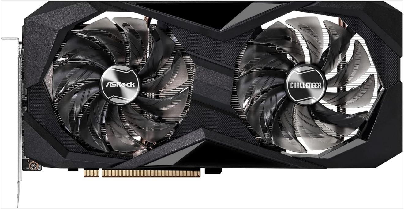
Figure 4.2: Front view of the ASRock RX 7600 Challenger graphics card, highlighting the dual fan design.
