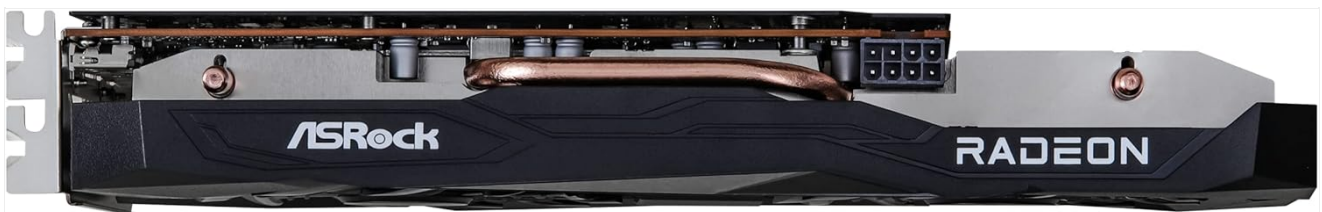
Figure 4.6: Side view of the ASRock RX 7600 Challenger graphics card, indicating the 8-pin power connector.
