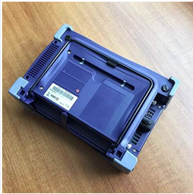
Image 5.2: Rear view of the MTS 6000 mainframe, illustrating the module bay for the E8126B OTDR module.
