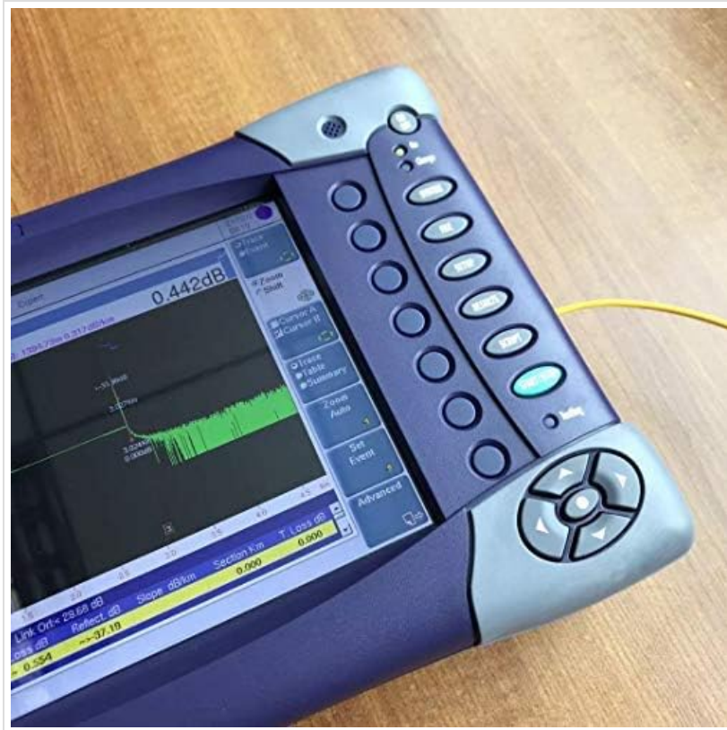
Image 6.1: A close-up of the MTS 6000 screen showing an active OTDR trace with event analysis.
