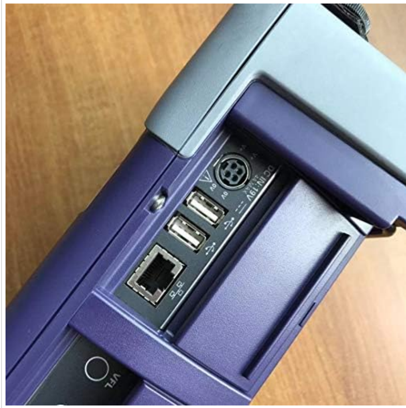
Image 4.3: Detailed view of the DC power input, USB ports, and Ethernet port.
