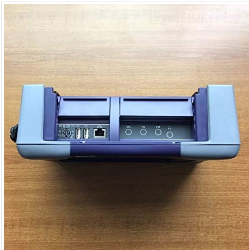
Image 4.2: Top view of the MTS 6000, highlighting the various input/output ports.
