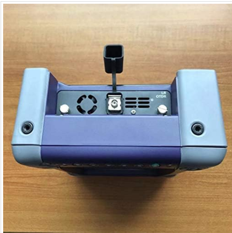
Image 4.4: Side view of the MTS 6000, showing the OTDR module port where fiber connections are made.
