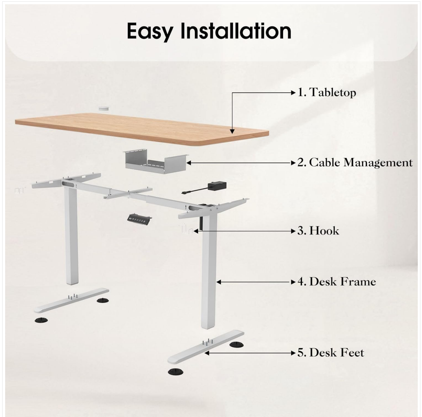
Image 2.1: Exploded diagram showing the main components of the desk: Tabletop, Cable Management, Hook, Desk Frame, and Desk Feet.
