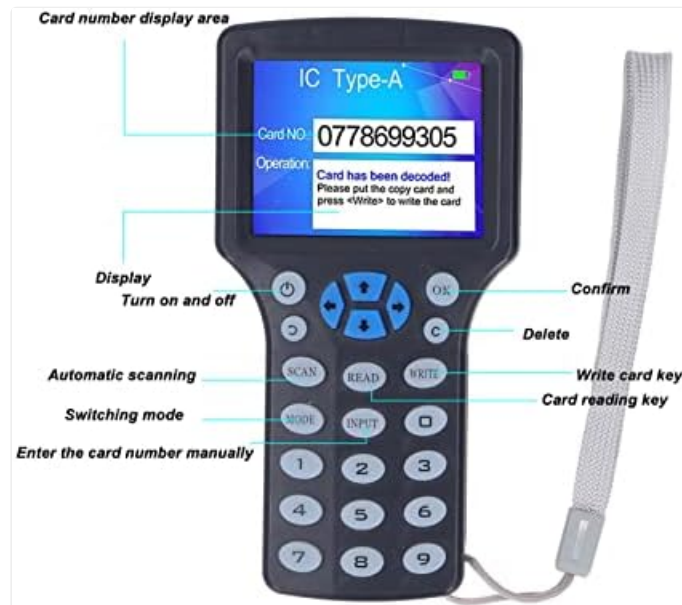
Figure 2.2: Labeled diagram of the copier's display and controls. Key elements include the display area, power button, OK button, delete button, scan button, read button, write button, mode switch, and input keys.
