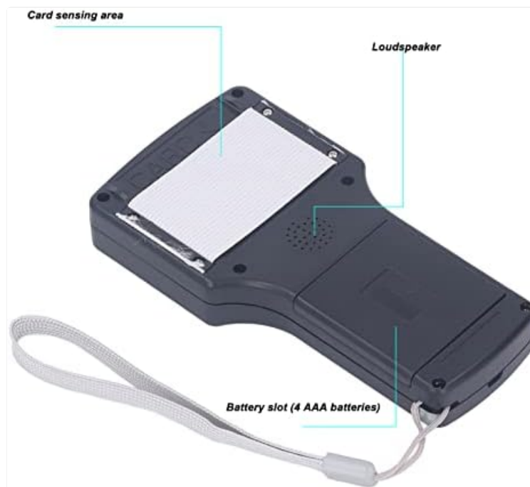
Figure 3.1: Rear view of the copier, highlighting the battery slot and card sensing area. The battery compartment is located on the back of the device.
