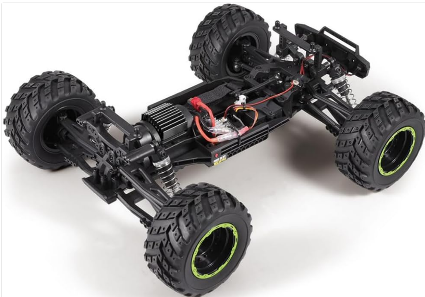
Figure 3.2: Chassis view of the BlackZon Smyter, showing battery and electronics placement.
