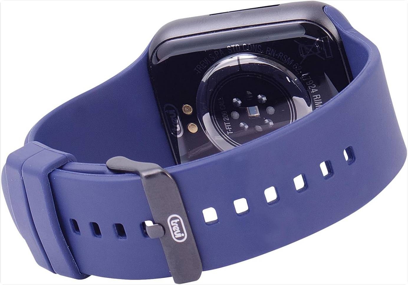
Figure 6.1: Detailed view of the smartwatch's rear, showing the optical sensors for health monitoring.
