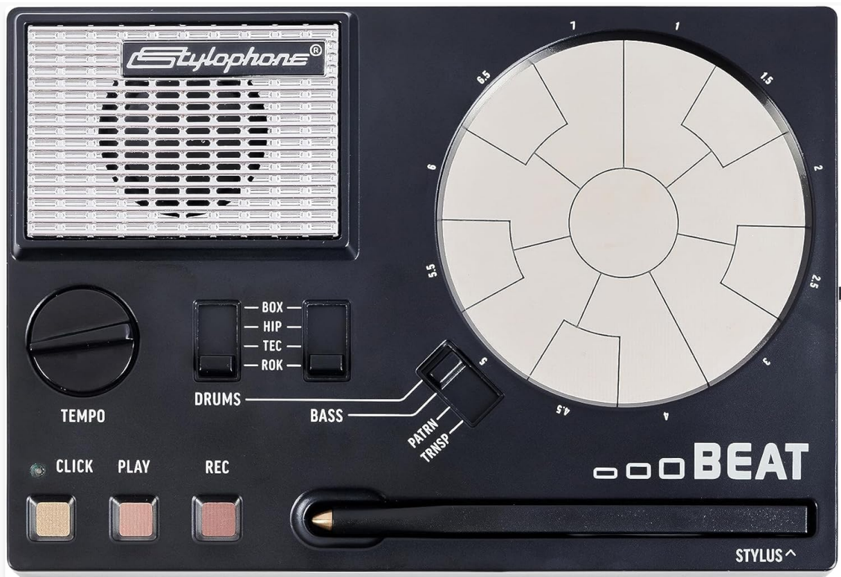
Image: An overhead view of the Stylophone Beat, clearly displaying the drum pad, drum kit selector, bass sound selector, tempo knob, and control buttons (Click, Play, Rec).
