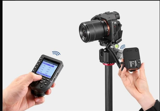
Trigger the camera shutter wirelessly. (Need to purchase NEEWER QR receiver & 2.5mm sync line separately)
