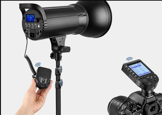
Use the 2.5mm sync interface to trigger non Q system flashes. (Need to purchase NEEWER QR receiver & 2.5mm sync line separately)
