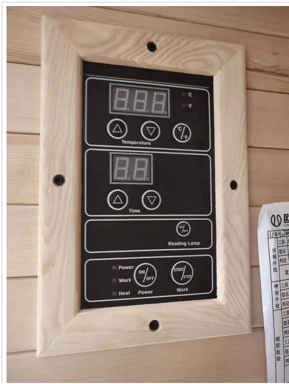
Figure 2.3: Interior control panel for adjusting temperature and time settings.
