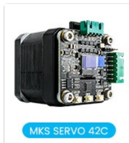
Figure 10: The board supports various driver modes including UART, SPI, and Normal STEP/DIR for flexible control.
