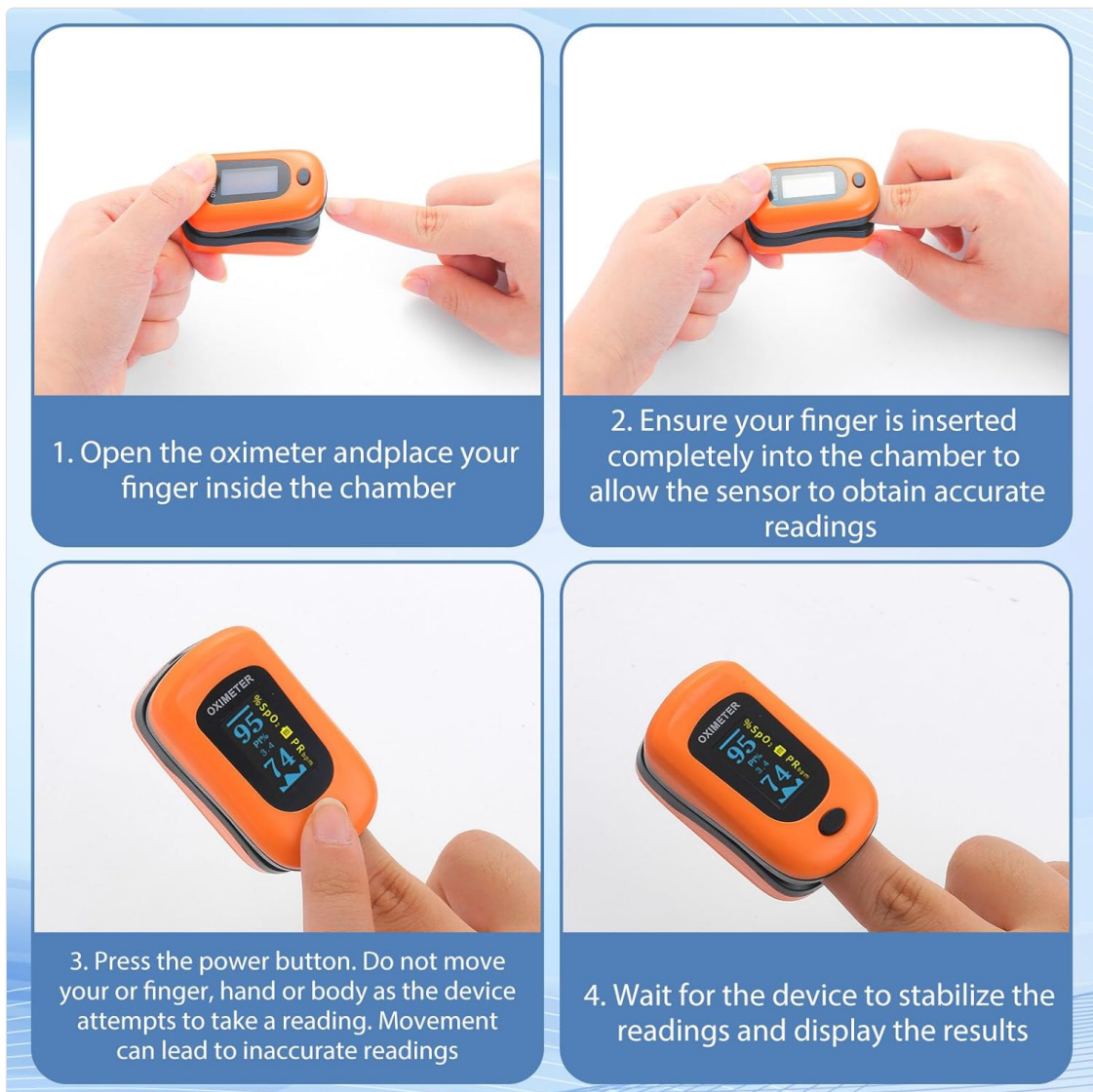
Figure 3: Step-by-step guide for using the pulse oximeter: 1. Open and insert finger. 2. Ensure full insertion. 3. Press power button and remain still. 4. Wait for results.
