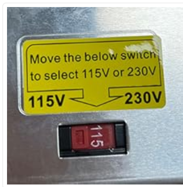
Figure 5.1: Input voltage selector switch. Ensure it matches your local power supply.
