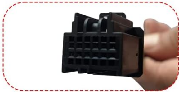
Image: Detail of the 12-pin extension cable, showing both male and female connectors.
