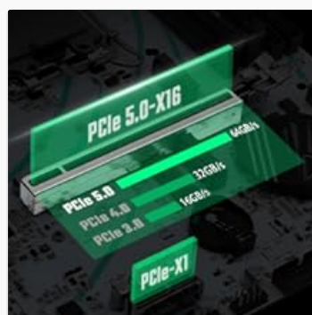
Figure 4.5: Diagram illustrating the bandwidth capabilities of PCIe 5.0 X16 (64GB/s), PCIe 4.0 (32GB/s), and PCIe 3.0 (16GB/s), highlighting the high-speed PCIe 5.0 X16 slot on the MACHINIST H610 motherboard.
