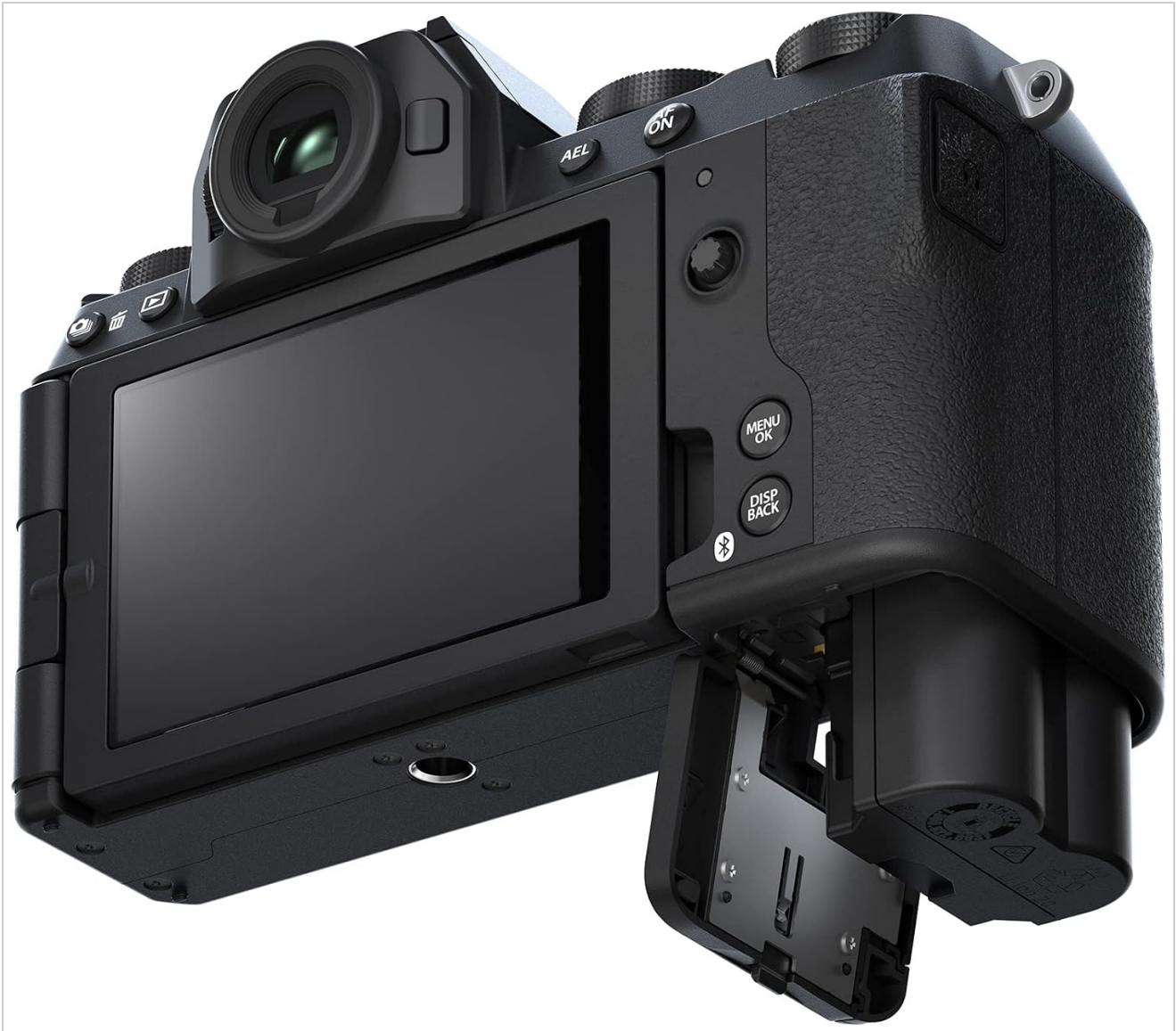
Figure 3.1: Battery and Memory Card Compartment. This image shows the bottom of the camera with the battery and memory card compartment open.
