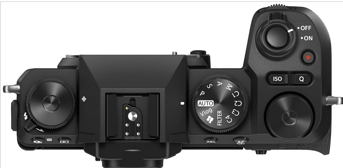
Figure 2.3: Top View of the Fujifilm X-S20. This image illustrates the top panel with the mode dial, shutter button, and other control dials.
