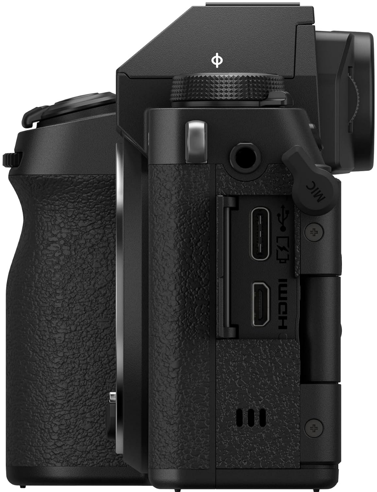
Figure 2.4: Side View of the Fujifilm X-S20 with Ports. This image shows the side of the camera, highlighting the USB-C, HDMI, and microphone ports.
