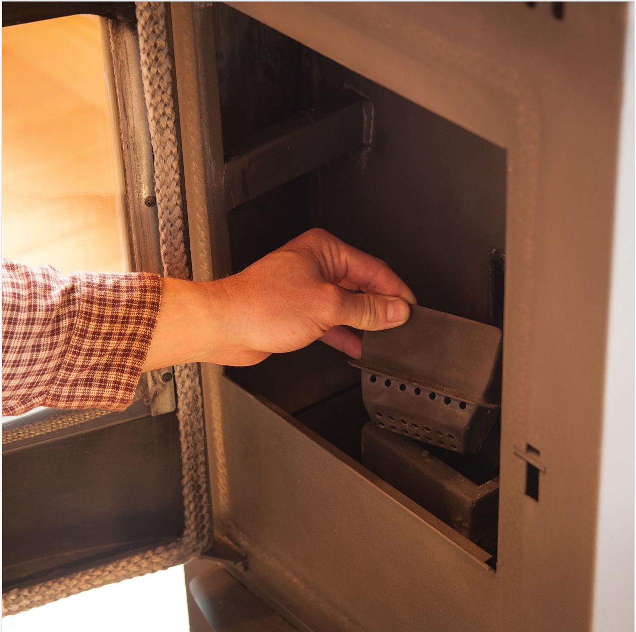
Figure 5: Removing the ash pot for cleaning.
