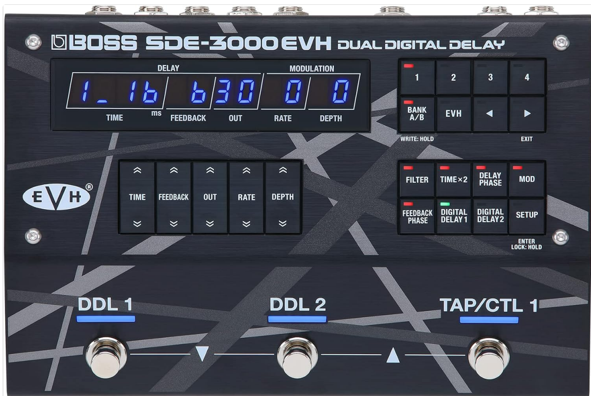
Figure 4: Top view of the SDE-3000EVH control panel.
