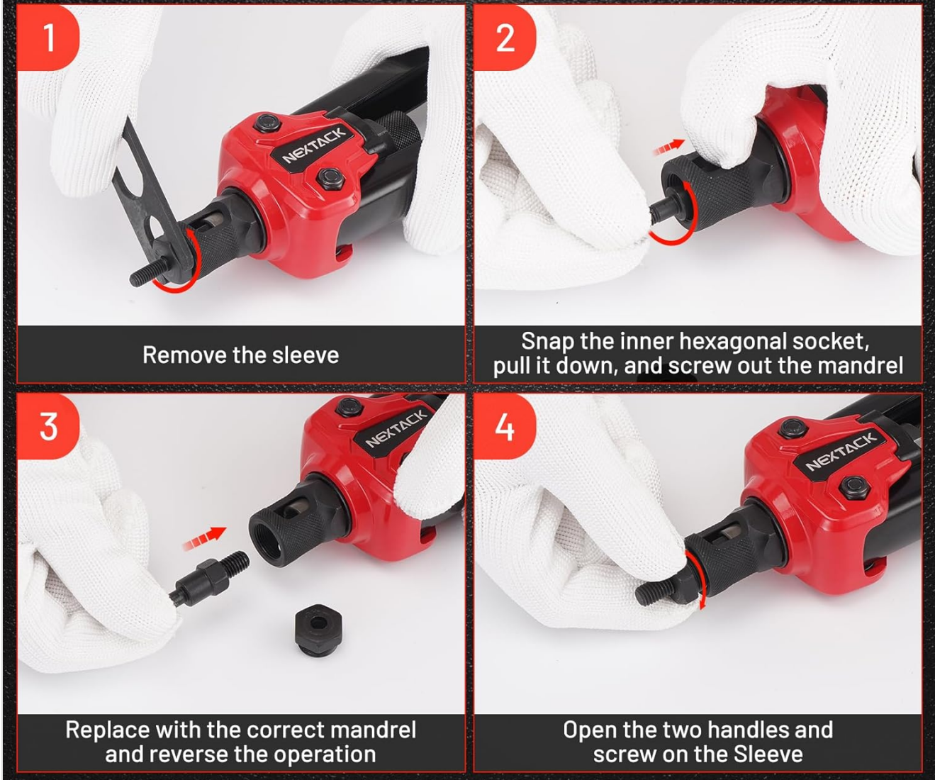
Figure 3: Visual guide illustrating the four steps for quickly changing mandrels on the NEXTACK NT700 rivnut tool.
