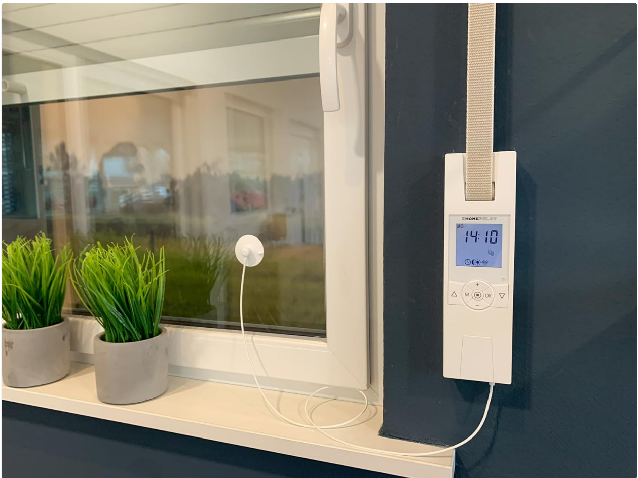
The HOMEPILOT Sun Sensor installed on a window, connected to a RolloTron belt winder.
