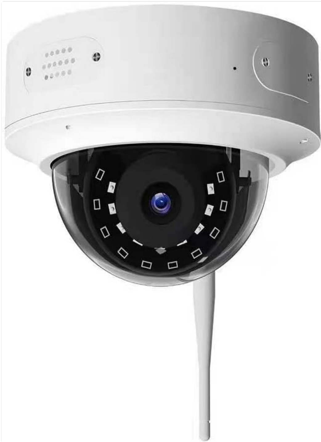
Figure 4.1: Front view of the Honistar 5MP Dome Camera, showing the lens, IR LEDs, and antenna. This camera is designed for integration into an existing surveillance system.
