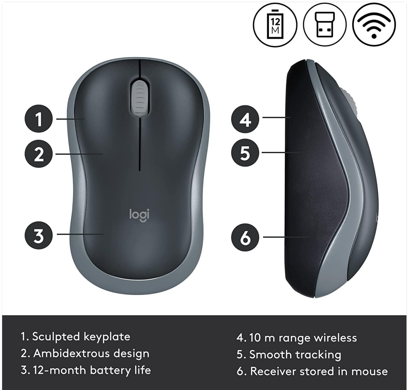
Figure 2.2: Detailed view of the Logitech M185 mouse highlighting its key features and components.
