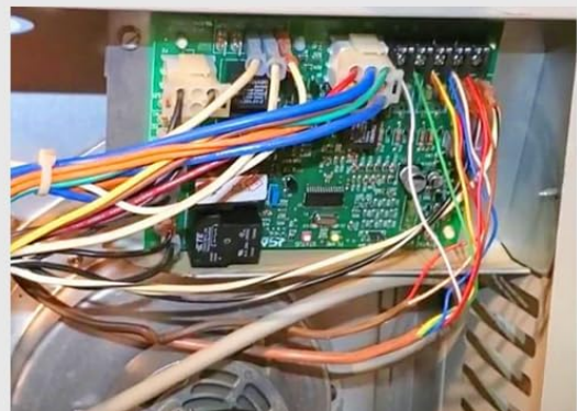
Image 2: Visual representation of the ICM2805A Control Board highlighting its broad compatibility.
