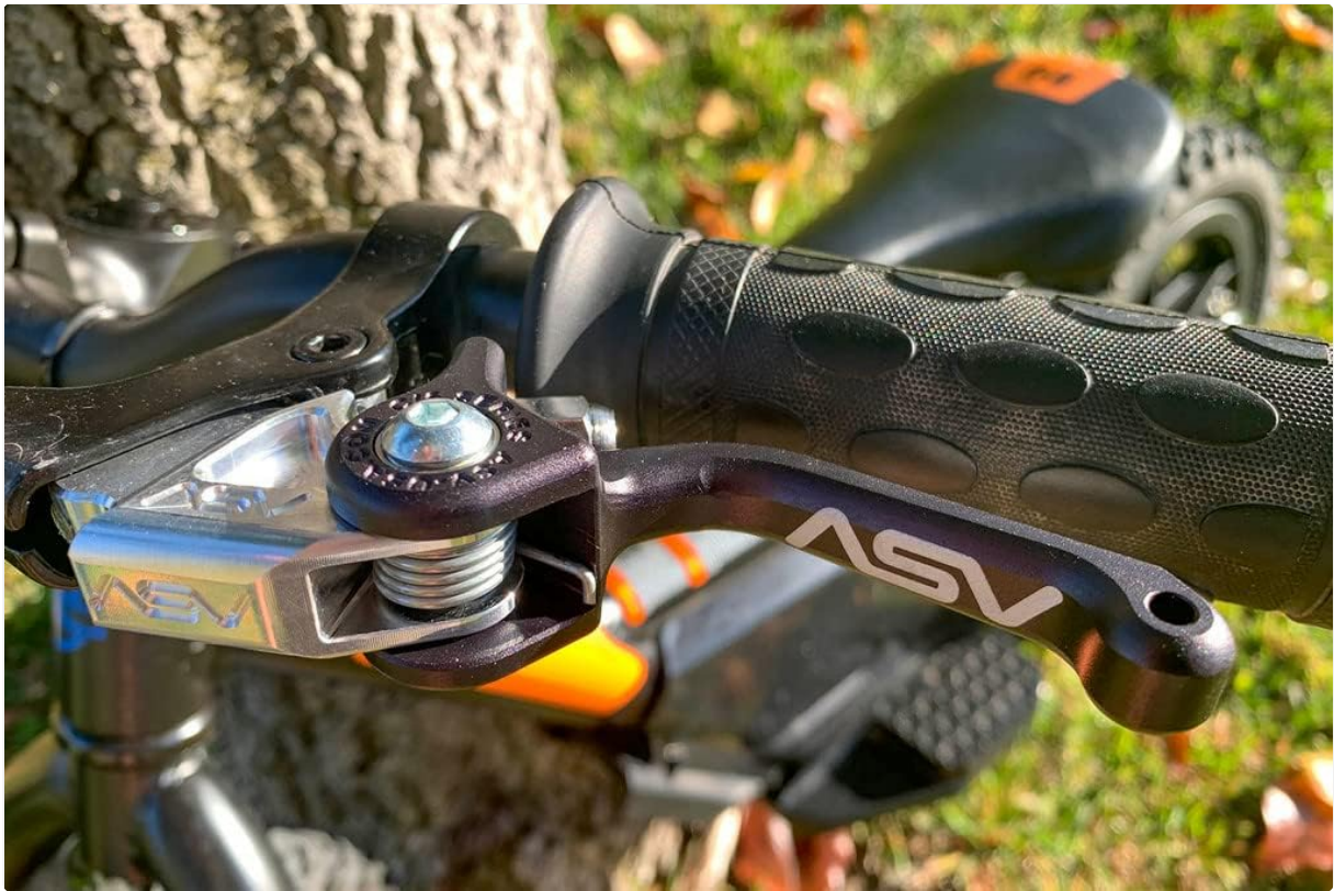
Image 2: The ASV F3 Series brake lever (black) installed on the handlebar of a Stacyc electric balance bike. This image demonstrates the lever's integration with the bike's controls.
