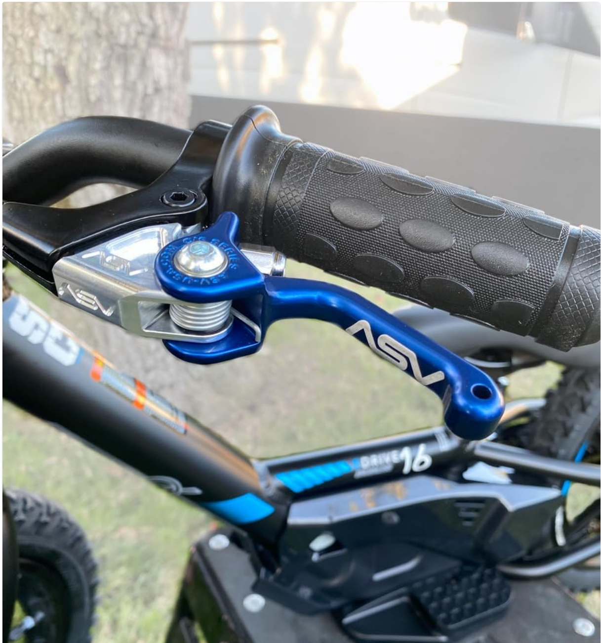
Image 3: A blue ASV F3 Series brake lever mounted on a Stacyc bike handlebar, illustrating the lever's position relative to the grip. This highlights the ergonomic design for easy access.
