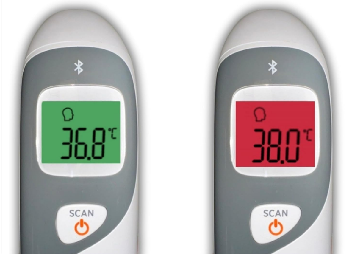
Image: The thermometer's color-changing LCD display indicating normal (green) and high (red) temperatures.
