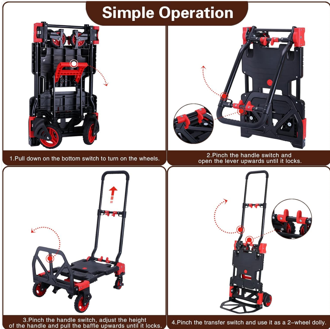
Figure 4.1: Step-by-step guide for unfolding and converting the hand truck.
