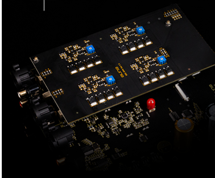
Figure 6: IIS Differential Transmission and Dual DAC Chip implementation.
