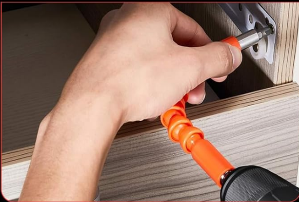
Figure 7: LED light in action, along with flexible shaft and drill brush applications.
