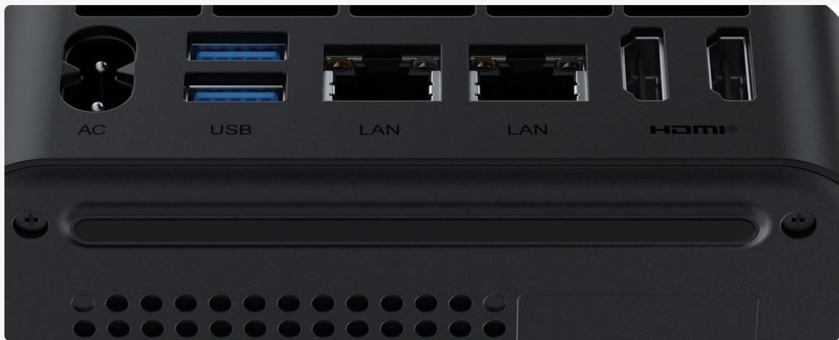
Figure 3: Close-up view of the Mini PC's ports, including AC power, USB, LAN, and HDMI.
