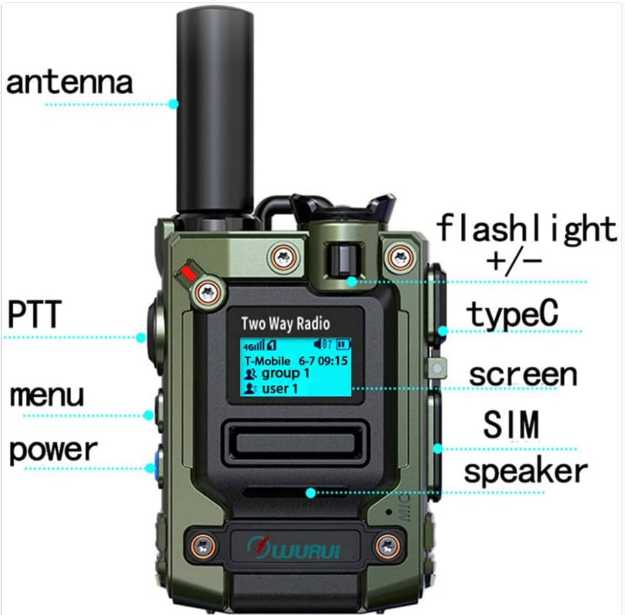
Image 3.1: Diagram illustrating the various controls and ports on the TXQ K300 radio.
