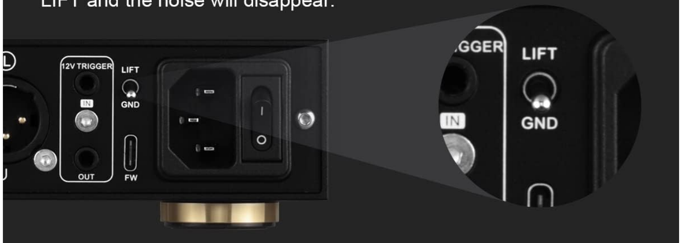
Image 5.1: Rear panel detail showing the GND/LIFT switch for ground loop noise reduction.
