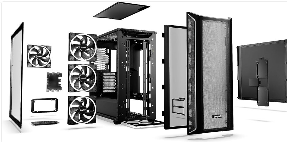
Figure 3.1: Exploded view showing the various removable components of the case, including panels, fans, and drive cages.
