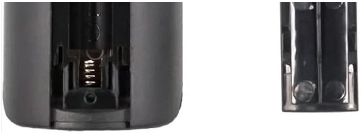
Image 2: Rear view of the remote control with the battery compartment open, showing where to insert AAA batteries.
