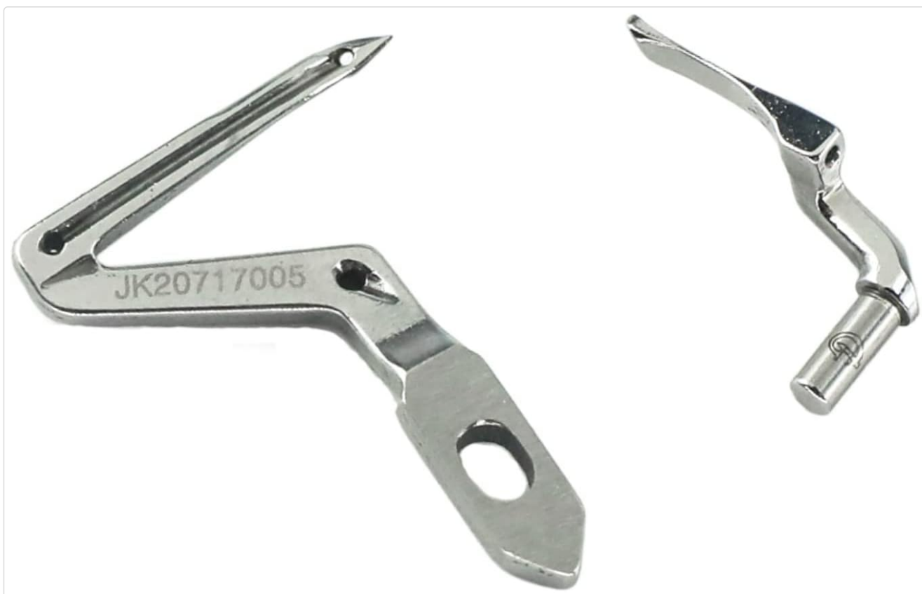
Figure 1: Blooy 20717004 Upper Looper and 20717005 Lower Looper shown together. These are critical components for forming stitches in an overlock sewing machine.
