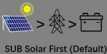
Figure 4.2: Visual representation of the four charging modes (CSO Solar First, Utility First, SNU Solar and Utility, OSO Only Solar) and three discharge modes (SUB Solar First, USB Utility First, SBU Priority).
