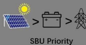
Figure 4.2: Visual representation of the four charging modes (CSO Solar First, Utility First, SNU Solar and Utility, OSO Only Solar) and three discharge modes (SUB Solar First, USB Utility First, SBU Priority).
