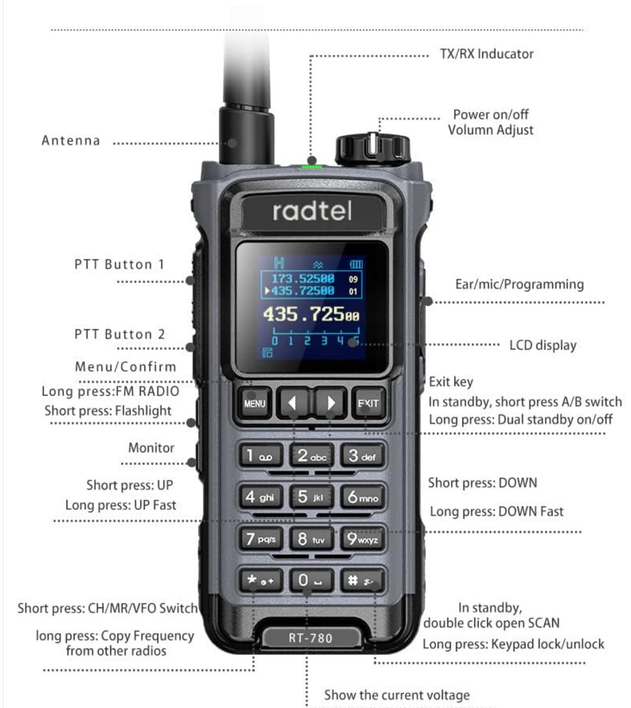
Figure 2: Radtel RT-780 Key Components and Controls
