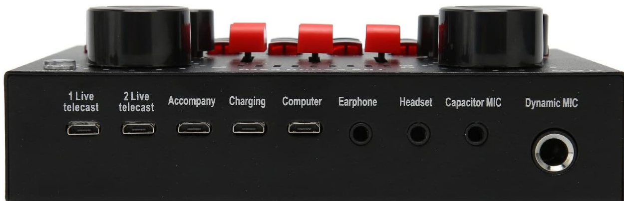
Image: The rear panel of the V8S sound card, displaying various USB, 3.5mm, and 6.35mm ports for connections.
