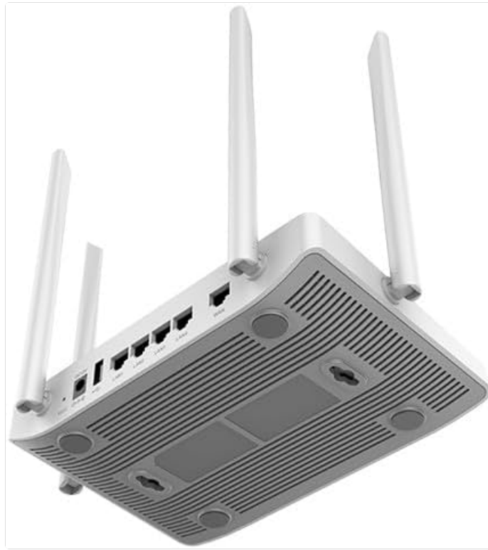
Image 2: Rear view of the GWN7052F router. This image highlights the various physical ports available on the back of the device, including the power input, WAN port, LAN ports, and a reset button.
