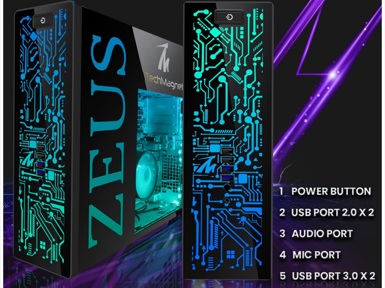
Image: Detailed view of the front panel ports on the Zeus PC tower, indicating locations for power, USB 2.0, audio, microphone, and USB 3.0 connections.
