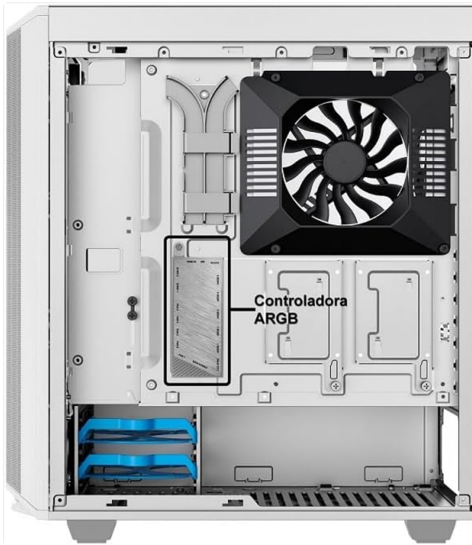
Figure 4.2: Rear internal view showing the ARGB controller for fan and lighting management.
