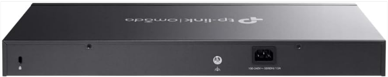
Image 2.3: Rear view of the TP-Link TL-SG3428X-M2 switch, showing the power input and grounding screw.
