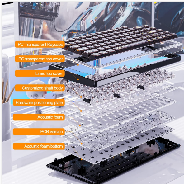
Figure 2.2: Exploded view illustrating the internal structure and layers of the K75 keyboard, including the gasket mount and acoustic foam.
